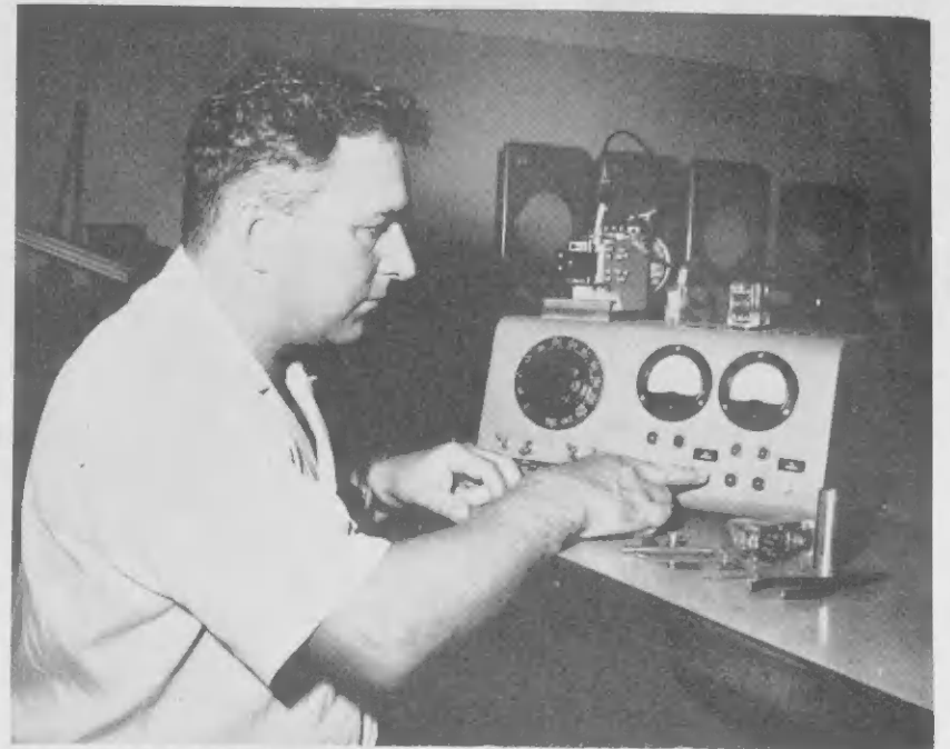
MAX SAND, technical assistant in the Instrument Shop, adjusts a control on the testing device he invented and designed for pretesting components for the lab's Automatic Standard Distillation Apparatus. For his Coin Your Idea, he was awarded Fls. 900 in April.
